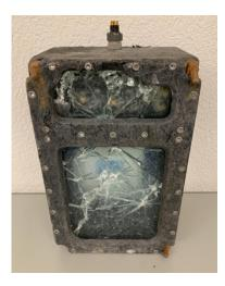
**Tough to the Core:** The camera housing was torn off a cliff face during a debris flow and retrieved from the debris collector below the installation site. The housing and safety glass were heavily damaged, but there was no water penetration into the housing, and the camera system is now back in operation in a new housing.
